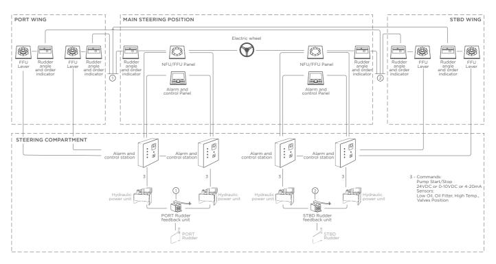
In the figure: two independent steering gears with two pumps in each gear is completely processed by represented ST5000 system on three steering positions.
